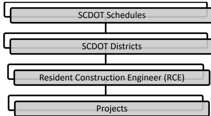
**Figure 3.3 Enterprise Project Structure of Primavera database**
